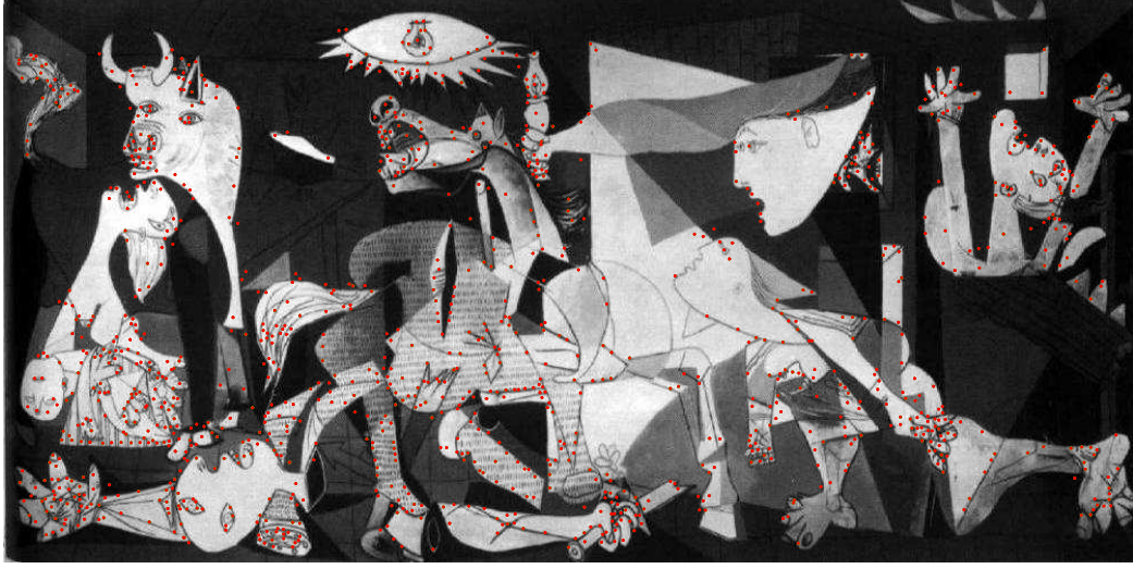
Figure 3.9: First 1200 points once detection by DoG has been made and also after having ordered the points according to their appearance in the different perspective images of the Guernica.
