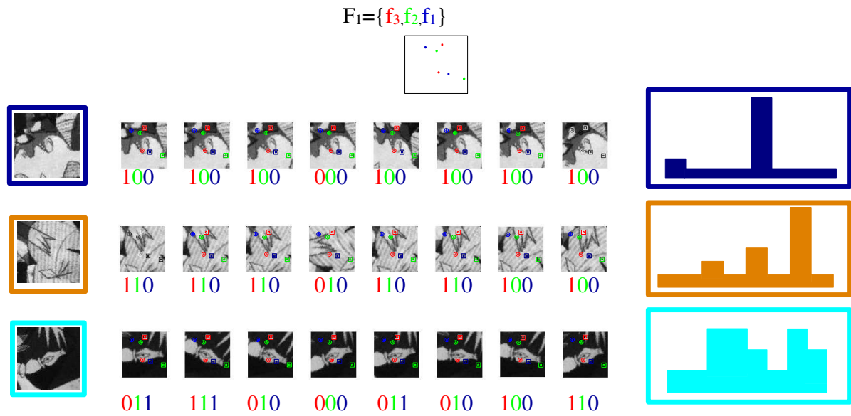
Figure 3.22: Probability distributions of fern F_1 conditioned to patches belonging to classes 1, 2 or 3 respectively ( P(F_1|k = \mathbf{k}_1) , P(F_1|k = \mathbf{k}_2) , P(F_1|k = \mathbf{k}_3) ).
