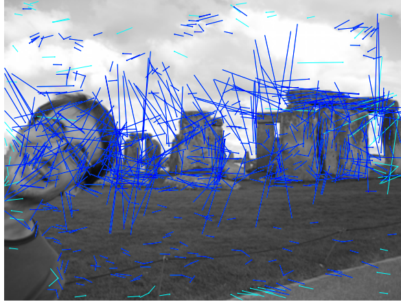
Figure 3.6: Set of detected points. Orientations are specified by vectors orientation which are born at the interest point location and which their magnitude is proportional to their gradient magnitude. In cyan, the points rejected after applying the edge criterion. In this image, initial set was of 738 points whereas, after eliminating boundary points, set had 669 elements.
