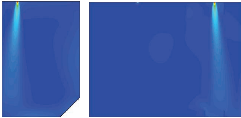
Figure 5.20 - Contour plots of velocity of planar slices through the jet inlet centreline; considerable off-axis jet bending is evident; Red represents 50m/s
