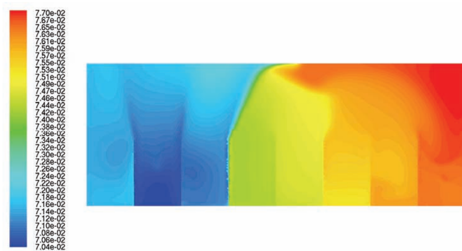
Figure 6.21 - Butane mass fraction on a vertical normal plane 0.1m above the floor; note the higher concentration in the outboard corner, top right
