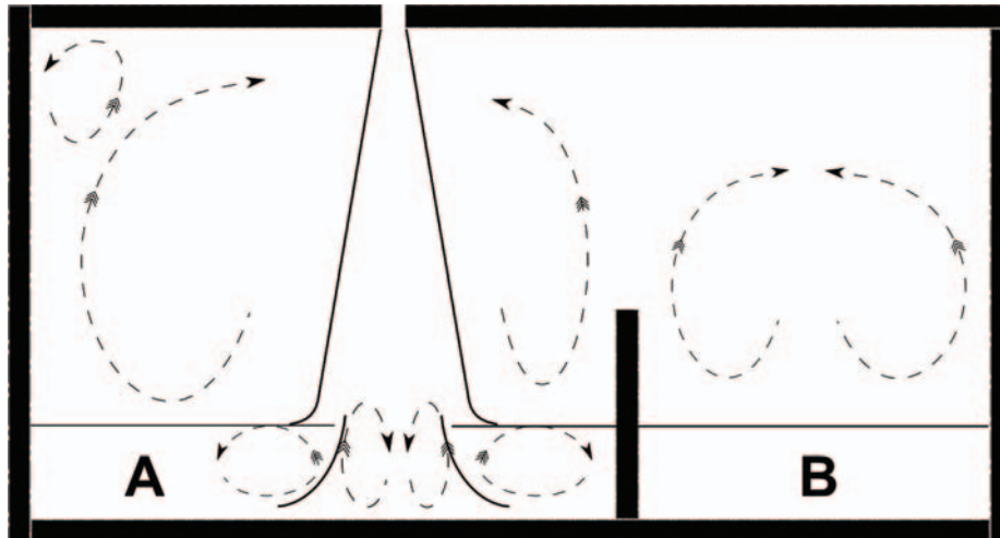
Figure 2.13 - Shear-induced recirculation flow patterns driven by a jet supply in an obstructed enclosure
