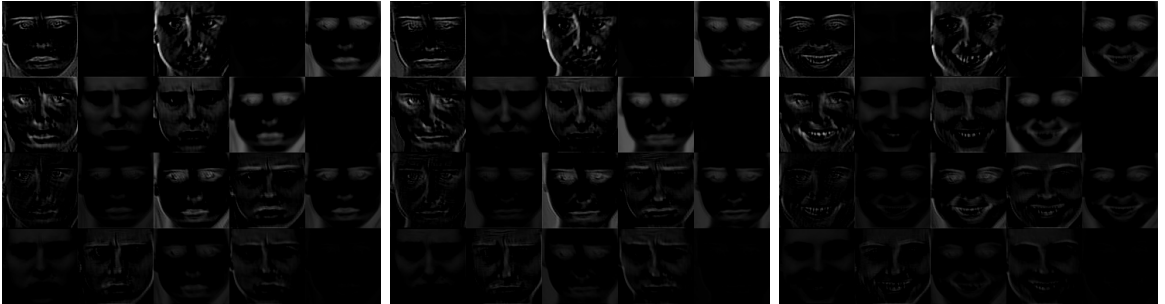
Figure 3.4: Sample visualization of filter kernels in the first convolutional layer. Left to right, subject F05 of the KDEF dataset illustrating: fear, sad, and happy emotions.
