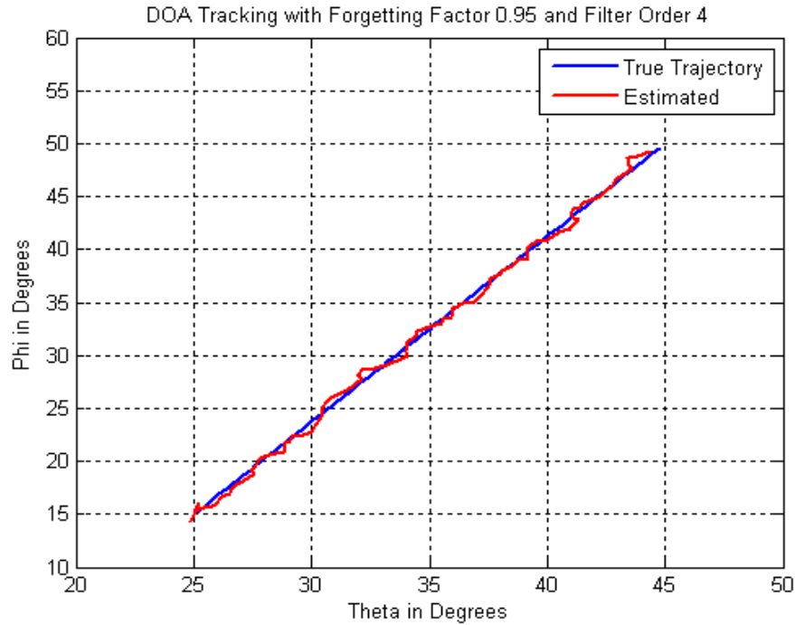
Figure 5.12: 2D-DOA Tracking with Orthogonal Polarized Planar Array with Forgetting Factor 0.95 and Filter Order 4, 20 dB SNR, \theta_{mse} = 0.0380 and \phi_{mse} = 0.0622
