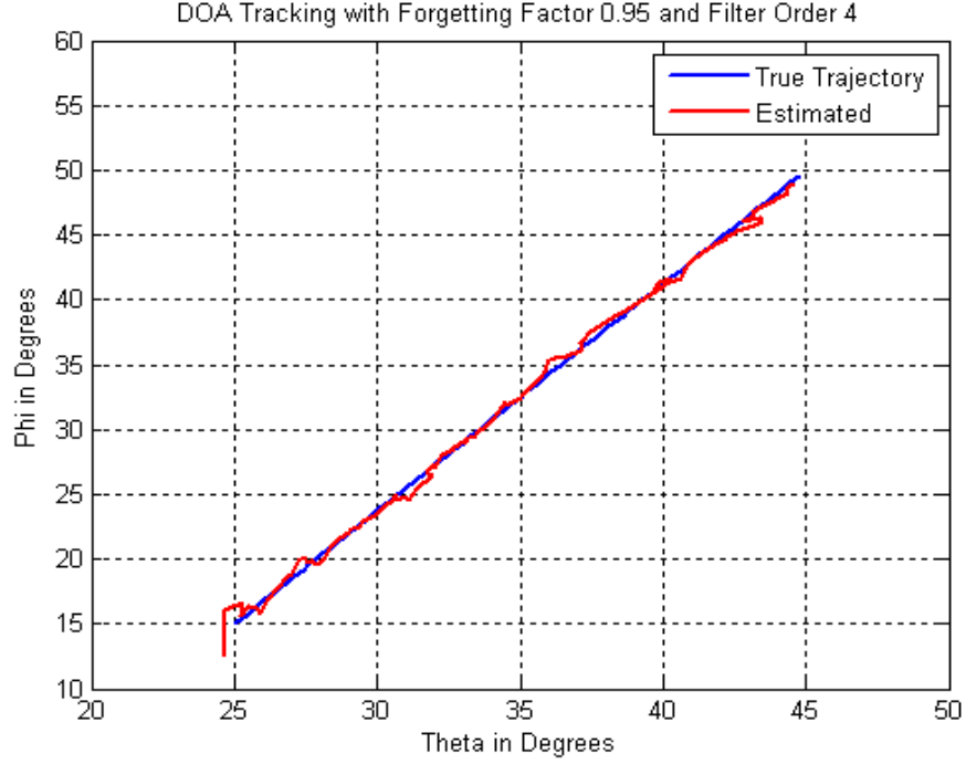
Figure 5.15: 2D-DOA Tracking with Orthogonal Mounted Linear Array with Forgetting Factor 20 dB SNR, \theta_{mse} = 0.0380 and \phi_{mse} = 0.0622
