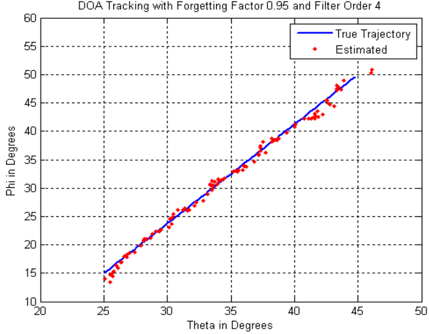
Figure 5.18: 2D-DOA Tracking with Orthogonal Polarized Linear Array with Forgetting Factor 20 dB SNR, \theta_{mse} = 0.0515 and \phi_{mse} = 0.0952
