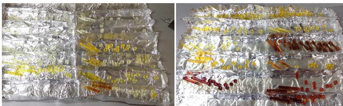
Figure 3-7. Photographs of assorted samples of all materials ( 3a1-4 ) after post-curing for 120 h at 120 °C in vacuo (left) and on air (right). Order of sample groups: 3a1, 3a2, 3b, 3c, 3d; 3a3, 3e1, 3e2, 3f1, 3f2, 4 (each downwards).
