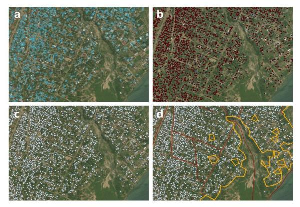
Figure 2-5 Built-up areas delineation process: a) Open Street Map buildings layer; b) Open Street Map buildings converted to points and checked/augmented; c) Building points buffered with a radius 4m; d) builtup areas delineated (yellow) as a function of building clusterings and inclusion of edge features (red)
