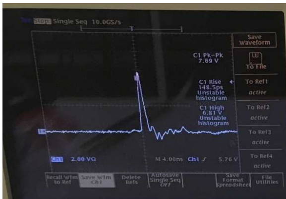
Fig. 10. Screenshot of an SRD generator output impulse when driven by G1. In this example, the observed risetime and amplitude were approximately 145 ps and 6.81 V respectively.
