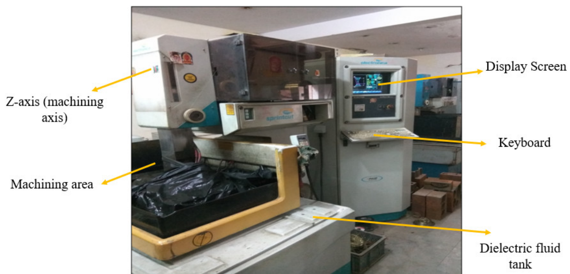
Figure 2. Pictorial view of the WEDM tool (courtesy: DIT University, Dehradun).
