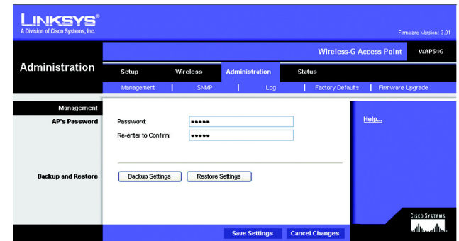
Figure 7-21: Administration - Management Screen
