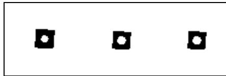
Fig. 5.31 From left to right: resulting marker, dilation 2x2 and dilation 3x3 of marker I5
