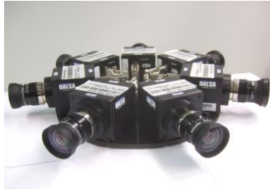
Fig. 1.4 Omnidirectional camera system
