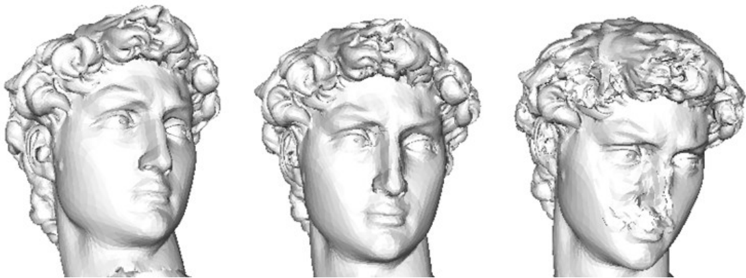
Figure 7.17. The original model and watermarked model with and without visual masking for the David Head model when using the same watermarking strength ( \Delta=0.9 ). From left to right, original David Head model, watermarked David Head model using the perceptual mask and watermarked David Head model without perceptual masking. We can observe that the perception of the watermark is more noticeable when we do not apply the visual mask. The watermarking strength have been selected so that the distortions due to watermark are visible.
