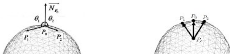
Fig. 6.2. From left to right: Calculation of curvature and roughness. (data courtesy of [DHM10])
