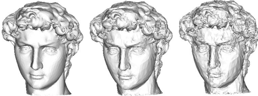
Figure 8.5. From left to right, original David Head model, the same model attacked with a Gaussian noise (NR = 0.002) and the model attacked with a more strong noise (NR = 0.004).
