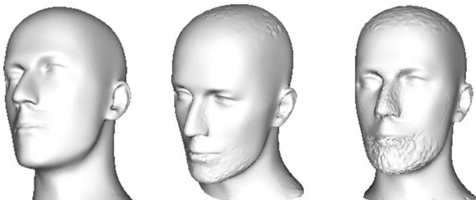
Figure 7.18. Same results than Fig. 7.17 for the Head model ( \Delta=0.2 ). As in Fig. 7.17, the difference when we do not apply the visual mask is noticeable. The watermarking strengths have been selected so that the distortions due to watermark are visible.
