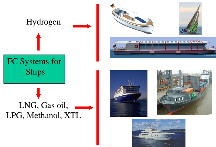
Figure 2: Which fuel for which application?
