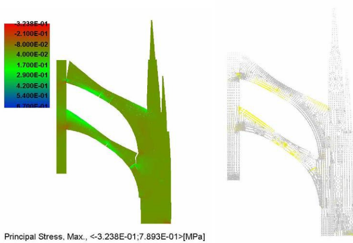
Figure 87 Model 2 Load history B a) Principal stresses b) Tensors
