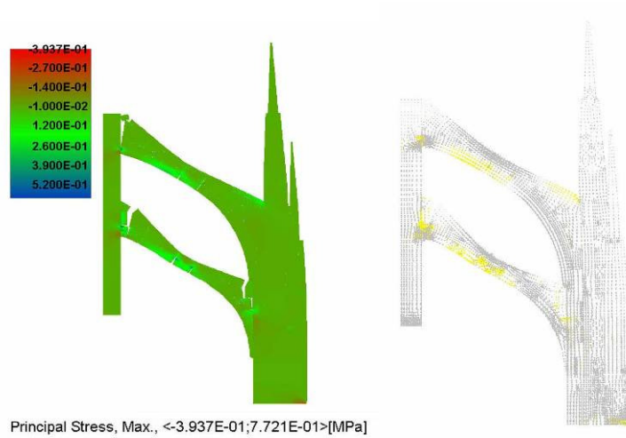
Figure 86 Model 2 Load history A a) Principal stresses b) Tensors
