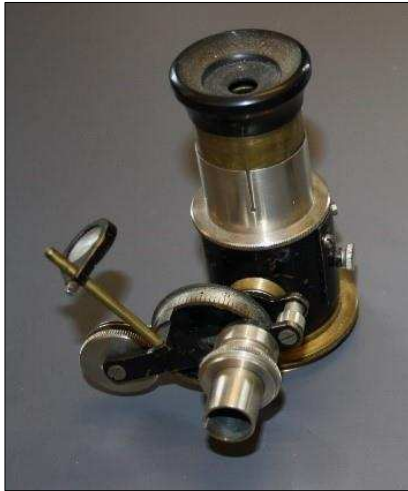
Figure 4: A ring micrometer (photograph: Bjørn Pettersen).
