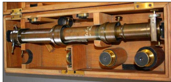
Figure 15: A Merz universal stellar spectroscope (photograph: Bjørn Pettersen).
