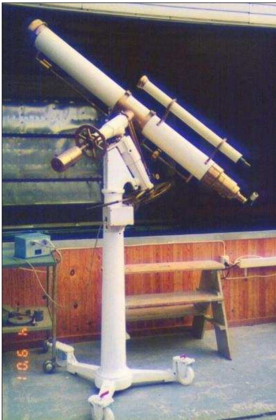
Figure 18: The 13-cm Merz refractor on an equatorial mounting by C.H.G. Olsen (photograph: Bjørn Pettersen).
