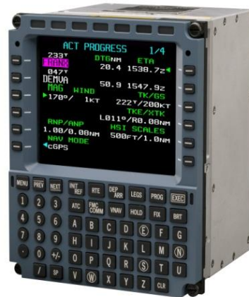
Figure 3.2 Control Display Unit (CDU)
