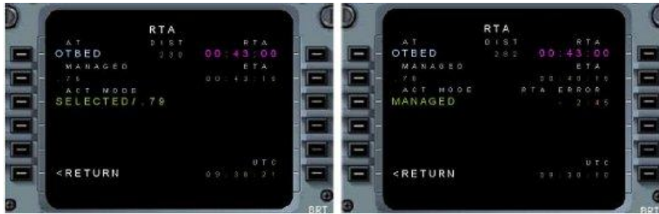
Figure 2.1: RTA function, in selected (left) and managed (right) speed modes [6]
