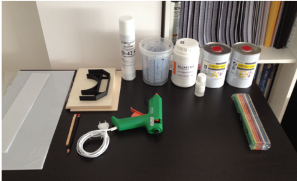
Figure 6.12 Material used for casting satellite shapes
