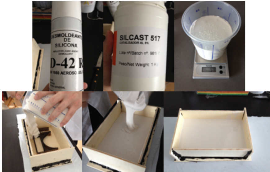
Figure 6.14 Casting of satellite shapes
