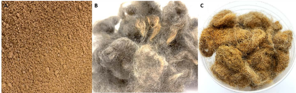
A) 50-Poly( S-r-canola ), B) Raw wool, C) Raw wool and 50-poly( S-r-canola ) mixture
