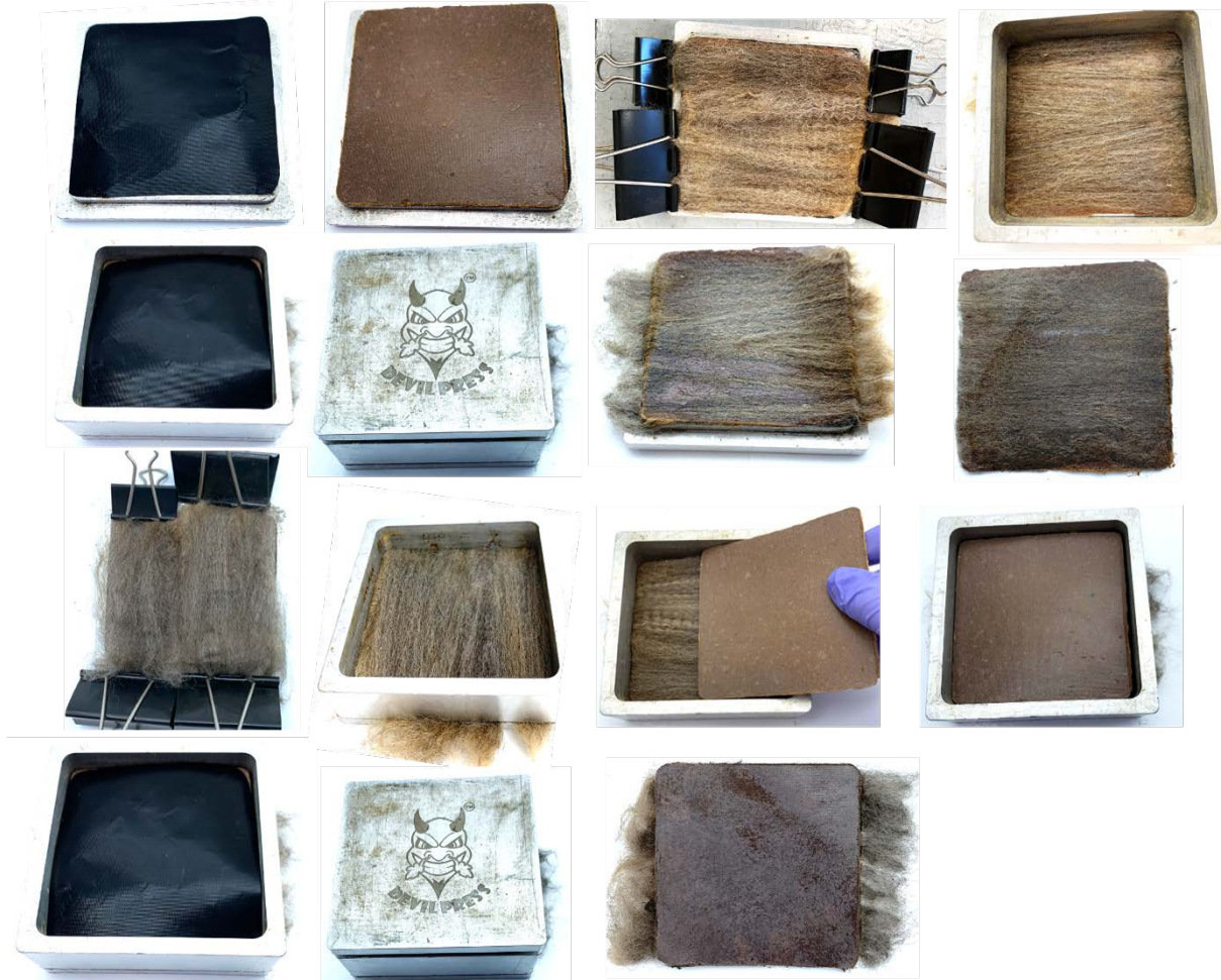
From left to right and top to bottom, images demonstrating the process used to prepare the composite mat with dual wool mats with orthogonal fiber alignment
