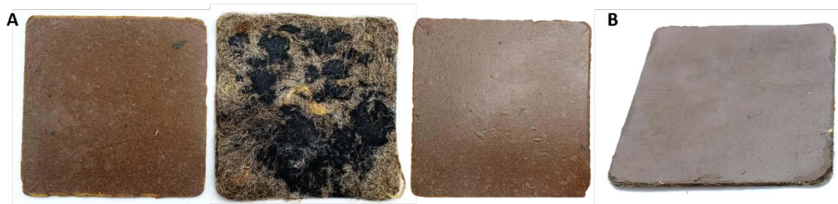
A) Two 50-poly( S-r-canola ) mats and one wool mat used in the preparation of the composite mat, B) Composite mat with one wool mat fixed between two 50-poly( S-r-canola ) mats using reactive compression molding.
