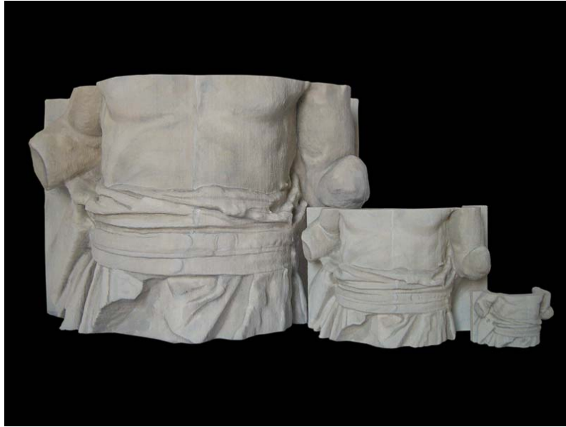
09 - By means of this procedure it is possible, starting from the same virtual model, to build solid models of any scale, from the full-size scale up to 1:5 scale, without losing in precision.
