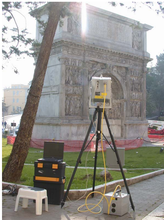
02 - The equipment for the survey included the 3D Cyrax 2500 laser scanner, a lap-top and a battery.
