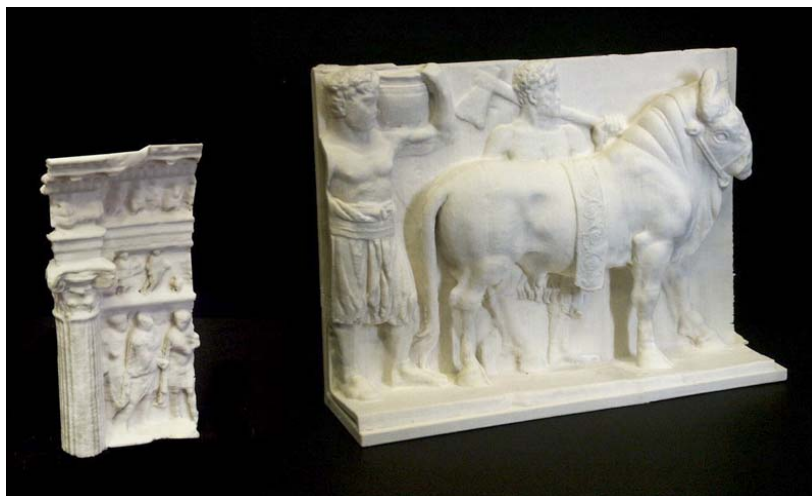
11 – The Cyrax data are suitable for the architectural scale prototyping, from 1:100 up to 1:20 scale.
