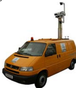
Figure 10: Multi-sensor system for façade documentation.
