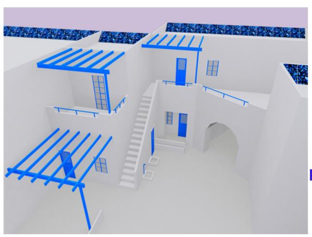
photovoltaic panels may be placed at the roof of the houses series of photovoltaic panels could be integrated to the pergola
