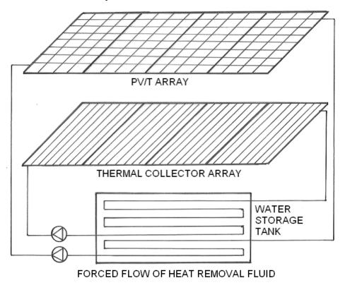
The flat plate solar thermal collectors are connected with the higher part of the water storage tank, to operate at higher temperature level of the system.
