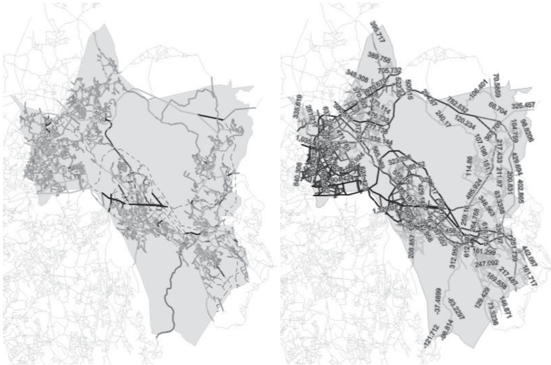
Figure 1: Two maps of the proposed plan showing the impact of the proposal. On the left the line intensity indicates an increase in global movement flow relative to the existing condition, with the dashed lines signalling new proposed roads. On the right are the forecasted traffic volumes of the proposal, with line intensity indicating higher numbers.
