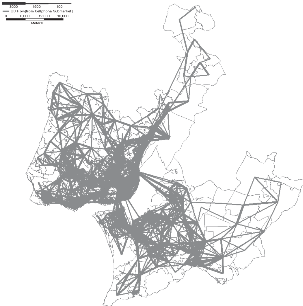
Figure 2: Average Daily ODs for all Trip Purposes in LMA as Estimated by Cell Phone Data
