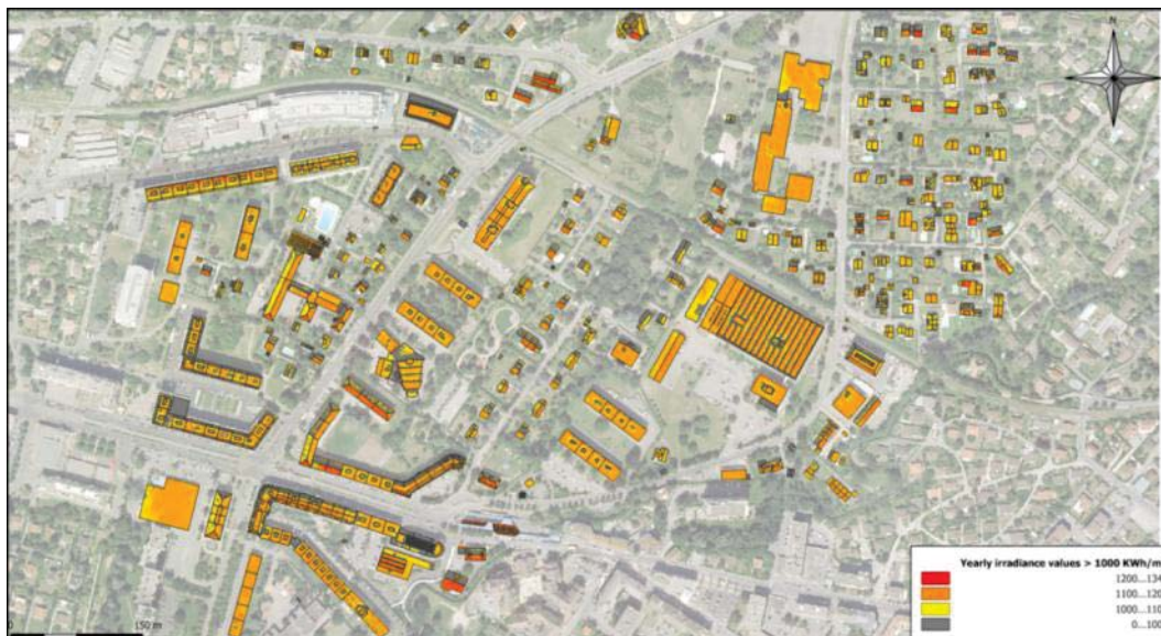
Figure 4: 2-D visualization of buildings using a LoD0 (projected in a 2-D view) considering a neighbourhood scale: quantitative indicator inherent to the yearly solar irradiation (KWh/m 2 ) by roof pixels for a neighbourhood (Moillesulaz pilot zone) of the city of Geneva.
