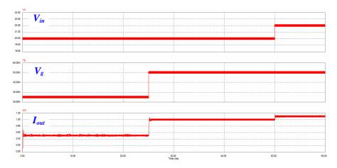
*Figure 8. Simulation results of the implemented G-type power gyrator.*
