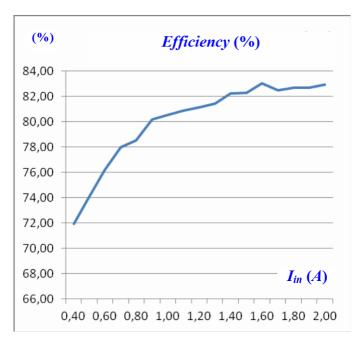
*Figure 7.* Experimental efficiency of the G-type power gyrator for different values of the input current.
