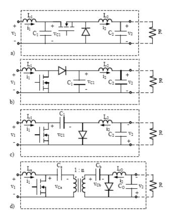
Figure 2. Classification of G-type power gyrators: (a) Buck with input filter (BIF), (b) boost with output filter (BOF), (c) Ćuk converter, and (d) Ćuk isolated.
