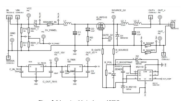
*Figure 5. Schematics of the implemented BIF G-type gyrator.*
