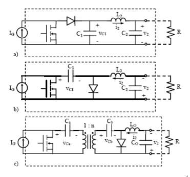
**Figure 4.** Classification of R-type gyrators: (a) boost with output filter (BOF), (b) Ćuk converter, and (c) Ćuk isolated.
