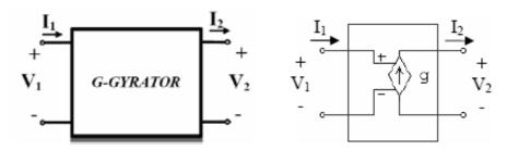
*Figure 1. Basic block of a* G-type power gyrator.
