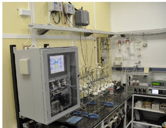
Fig. 3. On-line system of filtration of samples and analysis of nutrients and gases.
