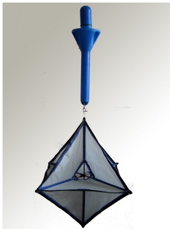
Figure 2. Lagrangian drifter equipped with a Davis-type drogue centered at 1 m depth.
