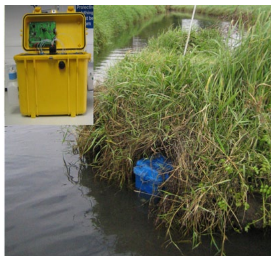
(right) Figure 2. Microfluidic based autonomous nutrient analyser.
