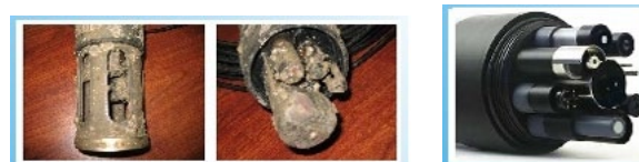
Fig. 3 Fouling in a classical buoy (left), clean sensors in Hidroboya (right)
