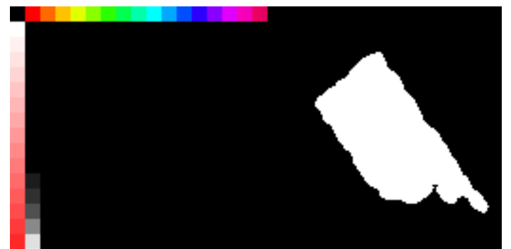
Fig. 2. The model of the target consists in a histogram of significant colours (left) and a shape (right).
