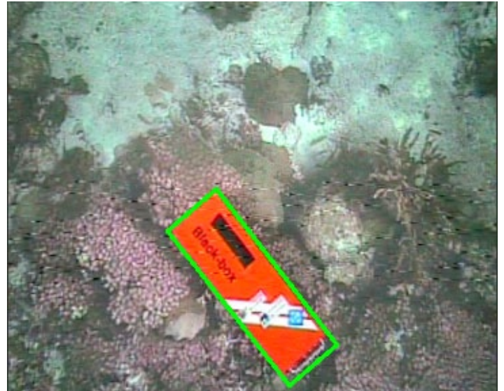
Fig. 1. Image taken by the AUV during the survey phase, labelled to train the system.
