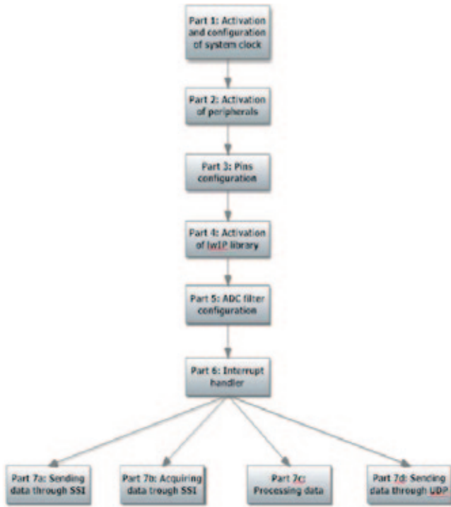
Figure 3: Flow-chart of main C program
