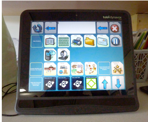
Fig. 1. Tobii Dynavox VOCA featuring Communicator 5 software with eye tracking access, photographed during the study.
