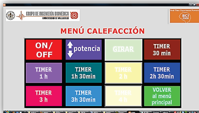
Figure 4. Heating Submenu of the domotic BCI application while running. The user can select different commands of the heater: on/off, timer, increase/decrease power, activate/deactivate the swing option, etc. In this frame the third column is highlight
