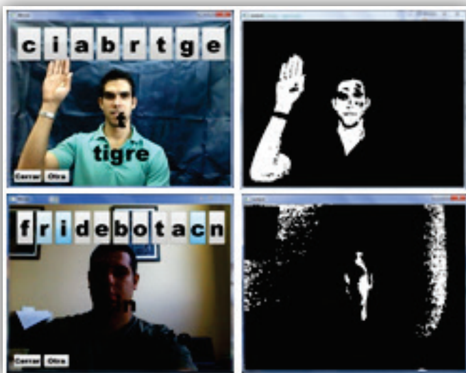
Figure 2. Skin Detection under different conditions. Source: University of Havana.
