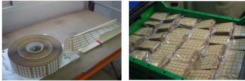
Figure 3. Poka-Yoke designed in WS3 (left) and end product to assemble (right)
