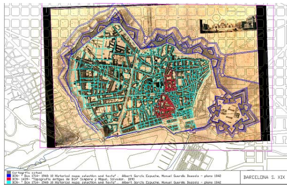
Figure I. Superposition of an 19 th century City Plan, adjusted and modified to meet the precision of today's cartographic plans.
