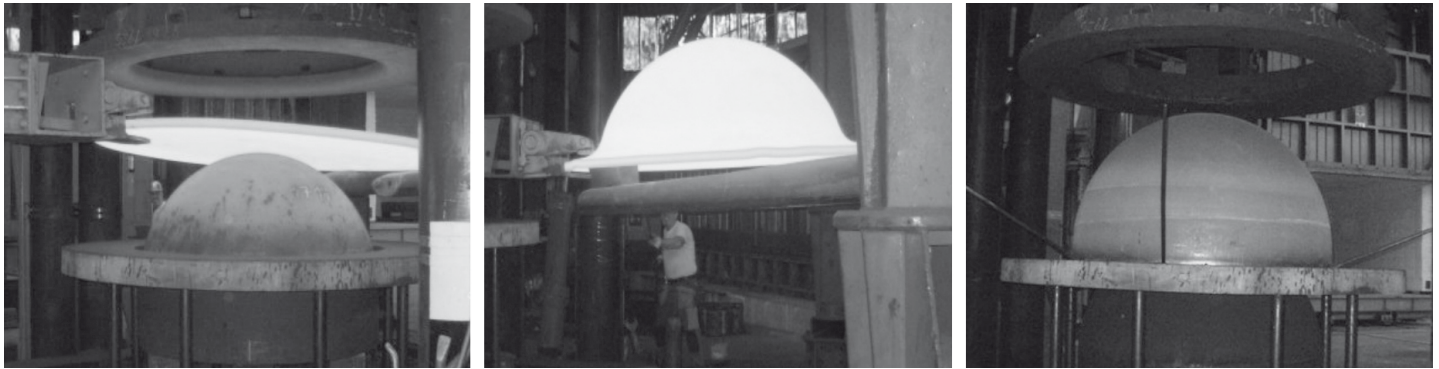
Fig. 2. Deep drawing of one hemispherical dished head
