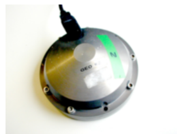
Figure 1. Structure of the coupling with triaxial geophones
