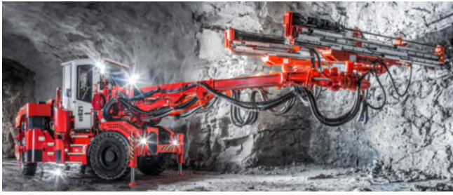
Fig. 1. A Sandvik tunneling jumbo with two drilling booms.
