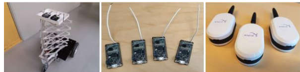
Fig. 6. Examples of mobile and stationary mMTC devices used in trials. The two left ones are LoRa and the right one NB-IoT devices.
