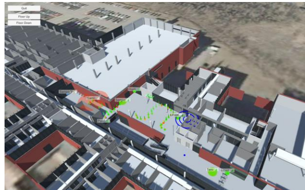
Fig. 5. A Unity based 3D visualization tool for assessing the performance of mobile mMTC sensors.
