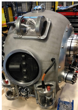
Fig. 14. UX-1 Complete pressure hull assembly
