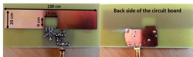
Fig. 6. Fabricated RF energy harvesting system.
