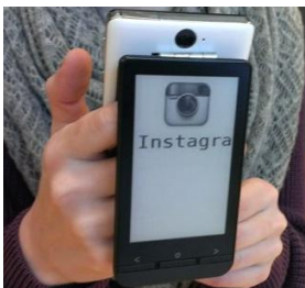
Figure 1. The Social Display revealing the user's currently used app to surrounding people.
