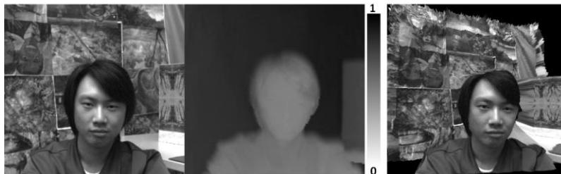
Fig. 3 Data fusion: view-plus-depth frame and 3D textured surface
