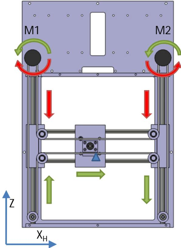
**Figure 4:** The H-Structure: XZ plane movements by M1&M2. View from front.
