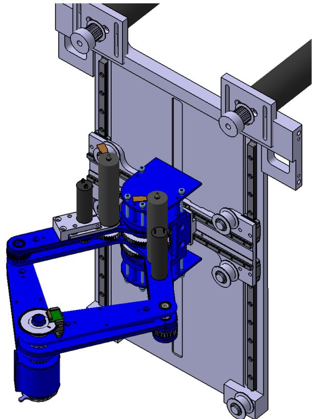
**Figure 2:** CAD-model of the H-scara manipulator. The belt driving the H-structure is not visible, only the belt pulleys.
