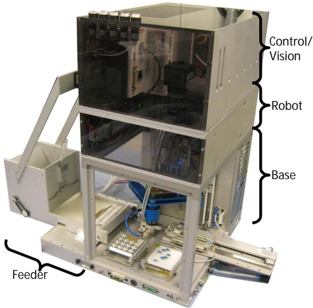
**Figure 1:** The assembly cell - H-Scara robot and feeder with the case product.
