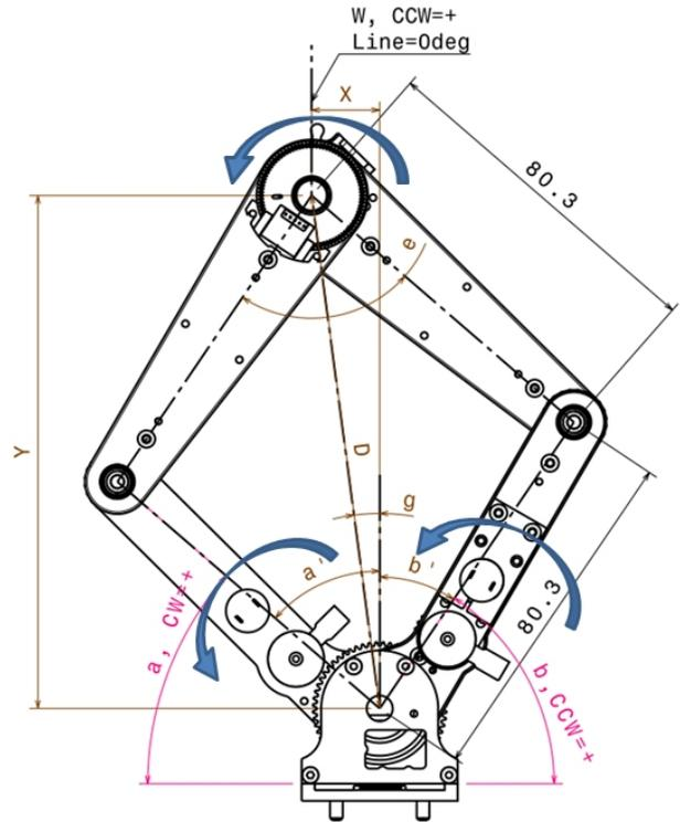
**Figure 5:** XY plane movements by parallel scara structure driven by the motors M3&M4. Illustrated is also the rotation of End effector (W-axis). View from top. Base located at bottom.
