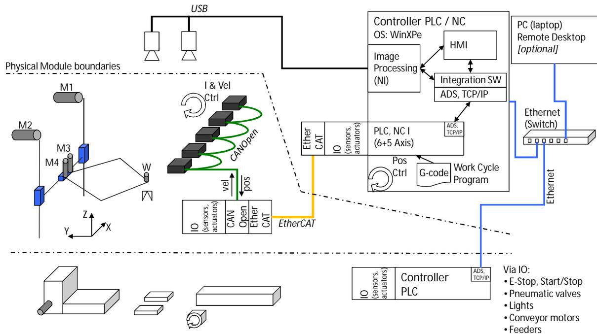
**Figure 6:** Control architecture of the cell.
