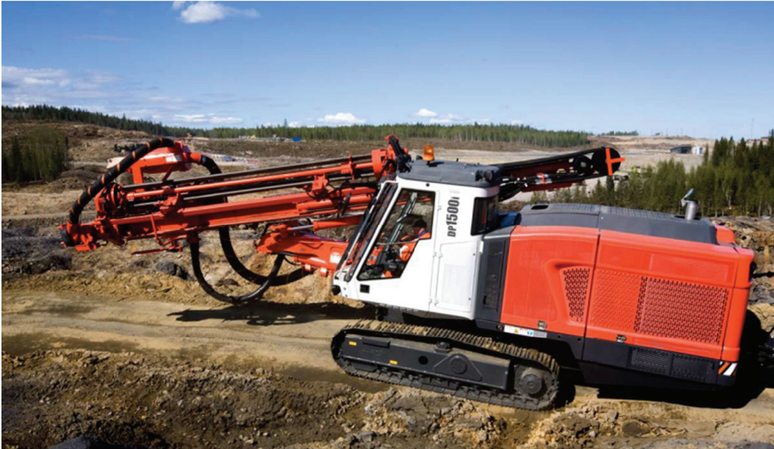
Figure 1. Surface top hammer drilling rig.[2]
