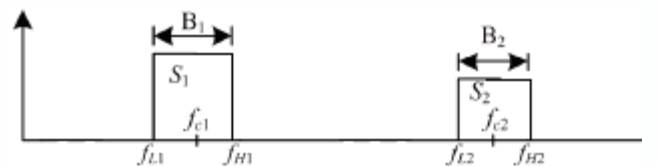
Fig. 4 Frequency spectrum of two complex RF signal bands
