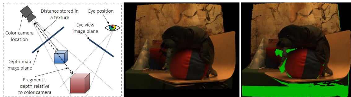
Figure 7. Occlusion detection results: a) occlusion detection scheme, b) no occlusion detection, erroneous color mapping, c) occlusions are detected, no texture assignment at occluded areas.
