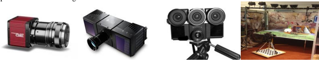
Figure 2. Camera setup: a) Prosilica GE 1900C, b) PMDTec CamCube 2.0, c) camera mounting setup, d) scene setup.
