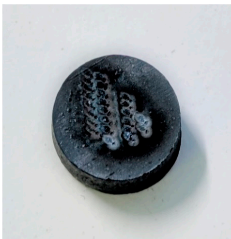
Figure 2. A pellet sample of 8 mm diameter was used as a sample for LIBS measurements.
