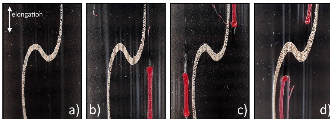
Figure 10. The area between two elongated meanders of the interconnect samples. (a) The unsupported meanders have elongated evenly from the tips of the meanders. (b) Bar supports between the meanders induce higher elongations in the meanders' tips. (c) Bar supports outside the meanders have changed the meanders' elongation. Close to the middles of the supports, the interconnects are denser and closer to the supports' edges and the interconnects have cracked more and thus elongated more. (d) Curved supports smooth the elongation of the interconnects and change the shapes of the elongated interconnects a little bit.
