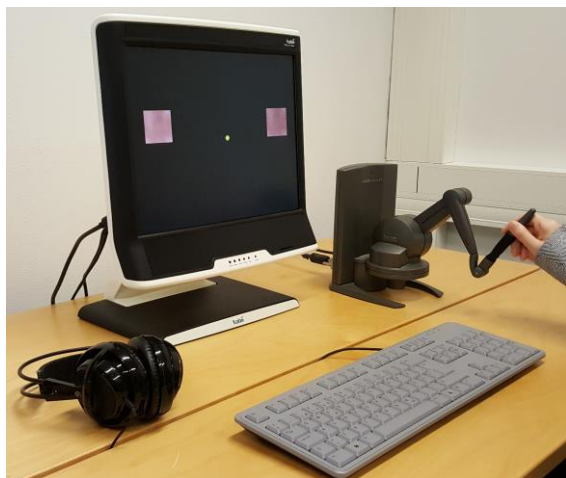
Figure 3: The experiment setup involved a Tobii T60 gaze tracker and a Phantom force-feedback device. The two skin models on the screen have the medium size of 4.8 cm (out of the three size levels) and the large distance of 24.3 cm between them (out of the three distance levels).
