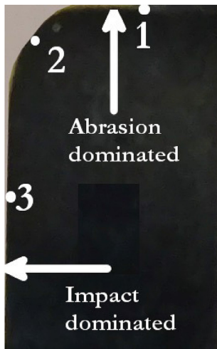
Fig. 13. The cross section sample 'B' shown in Fig. 13 of the impact-tumbler sample. Abrasion predominates in region '1', and impact damage in regions '3', with region '2' representing a transition area.
